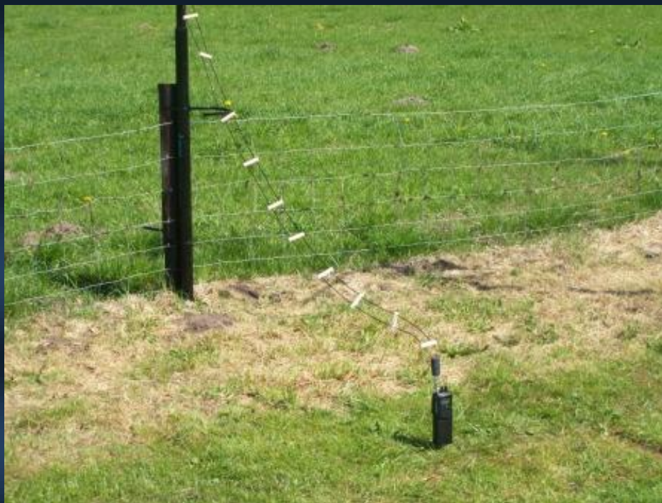
And the home made open lint line (quarter wave transformer)
